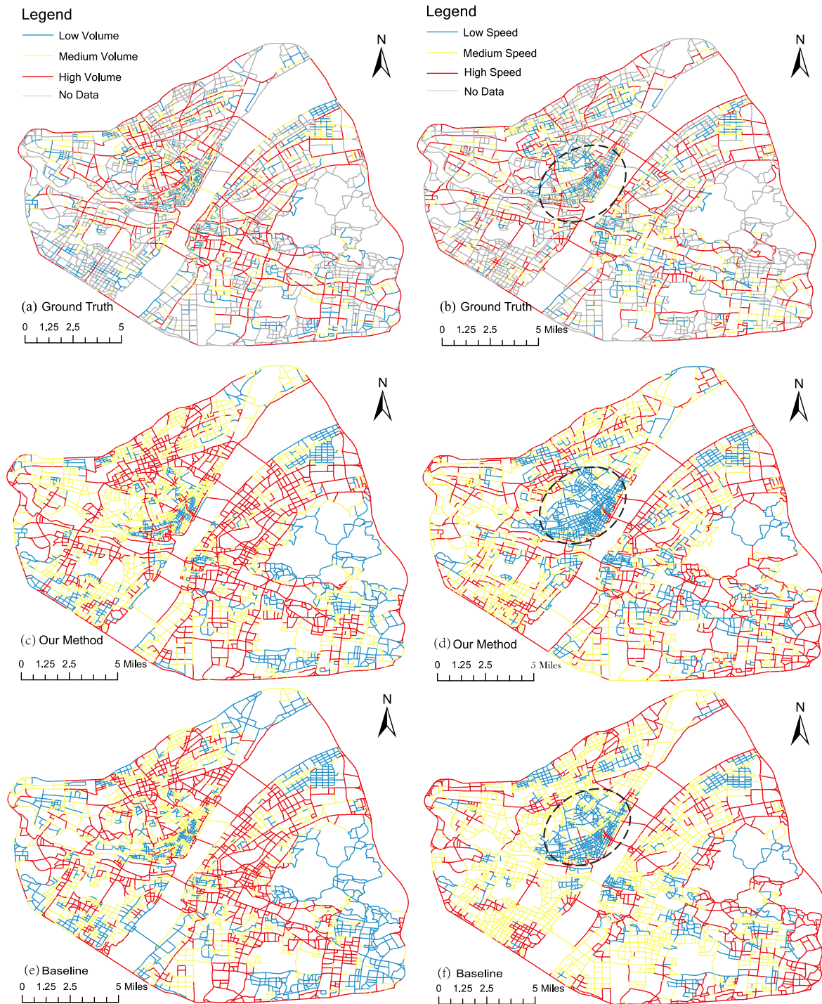
Fig. 9. Comparative visualization of traffic flow volume and speed predictions. Panels (a) and (c) illustrate the ground truth of traffic flow volume and speed. Panels (c) and (d) illustrate the predicted distribution of traffic volume and speed, respectively, after accounting for long-distance spatial interactions. Panels (e) and (f) showcase the spatial distribution of predicted values when the model considers only near-range spatial dependencies. This figure emphasizes the enhanced predictive accuracy in most areas when long-distance spatial interactions are integrated into the model. It particularly highlights the marked decrease in predicted road section flow speeds (panels (d) and (f)) and the significant increase in traffic volume predictions (panels (c) and (e)) in urban core areas, underscoring the potential limitations of traditional traffic forecasting methods in high-density urban zones.
