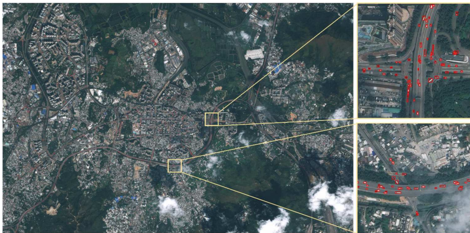
Figure 7. Vehicle Detection Visual Results (Based on the detected vehicle locations, we can match them to the nearest roads and compute the road density at this time).
